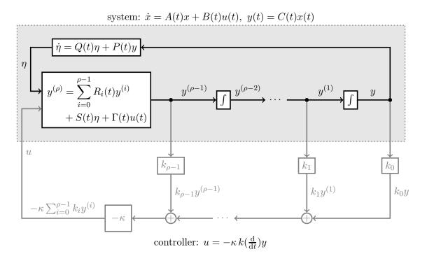
Figure 1: Byrnes-Isidori form and derivative output feedback controller
