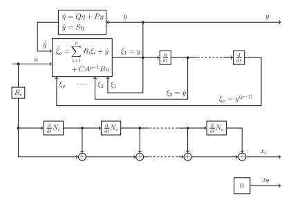
Figure 5.6: Zero dynamics form for systems with positive strict relative degree
