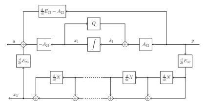
Figure 4.1: System  $[E, A, B, C] \in \Sigma_{l,n,m,p}$  in form (4.2.3)
