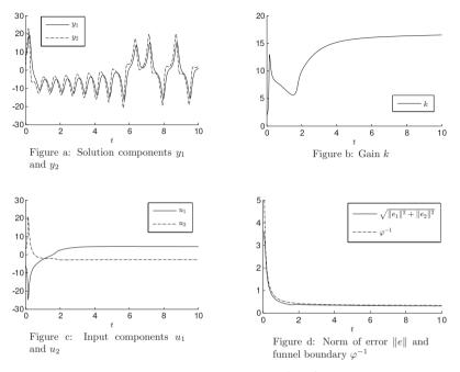
Figure 5.5: Simulation of the funnel controller (5.2.2) with funnel boundary specified in (5.2.22) and reference signal  $y_{\text{ref}} = (\xi_1, \xi_2)^{\top}$ given in (5.2.21) applied to system (5.2.24) with initial data (5.2.25), (5.2.26).
