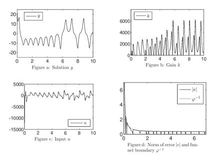
Figure 5.7: Velocity control: Simulation of the funnel controller (5.3.20) with funnel boundary specified in (5.2.22) and reference signal  $y_{ref} = \xi_1$ given in (5.2.21) applied to the mechanical model (5.3.23) with data (5.2.23), (5.3.25).
