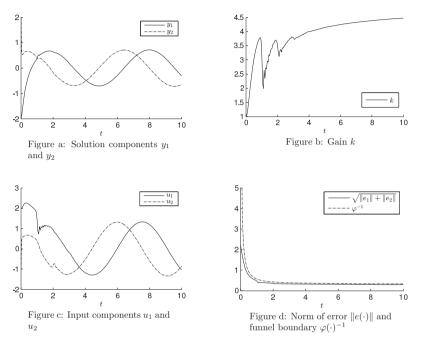
Figure 6.3: Simulation of the funnel controller (6.6.1) with funnel boundary specified in (6.7.2) and reference signal  $y_{\text{ref}} = (\sin, \cos)^{\top}$  applied to system [E, A, B, C] with initial data (6.7.1).
