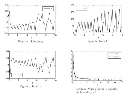
Figure 5.4: Simulation of the funnel controller (5.2.2) with funnel boundary specified in (5.2.22) and reference signal  $y_{ref} = \xi_1$  given in (5.2.21) applied to the mechanical model (5.2.18) with data (5.2.23).
