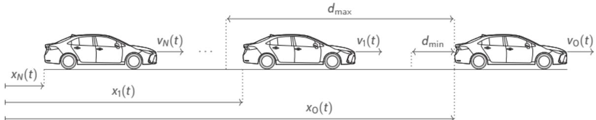
$$\begin{aligned}\dot{x}_i(t) &= v_i(t), \\ m_i \dot{v}_i(t) &= u_i(t) - f_i(t, x_i(t), v_i(t)) + d_i(t), \quad i = 1, \dots, N\end{aligned}$$
