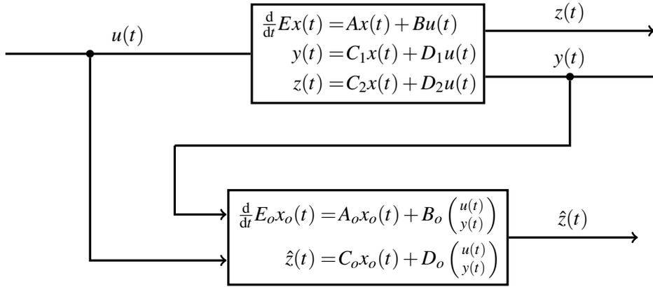
Figure 2.: Interconnection with an acceptor
