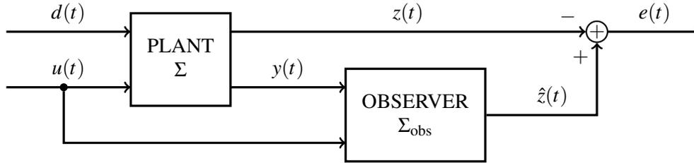
Figure 1.: Interconnection of plant and observer
