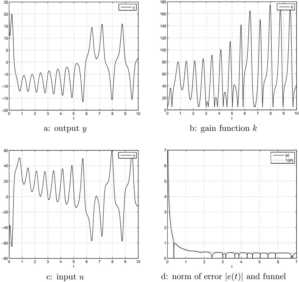
Figure 5: Simulation of the funnel controller (6.3) with funnel boundary specified in (7.2) and reference signal  $y_{\text{ref}}(\cdot) = \xi_1(\cdot)$  given in (7.1) applied to the mechanical model (7.3) with data (7.5).
