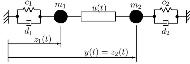
Figure 4: Mass-spring-damper system
