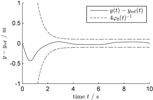
Fig. 11 a: Funnel and tracking error
