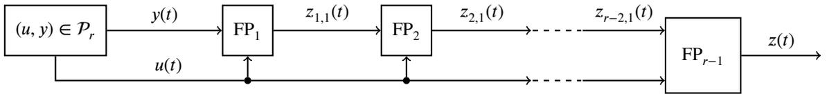
**FIGURE 4** Cascade of funnel pre-compensators (1) applied to signals  $(u, y) \in \mathcal{P}_r$ .
