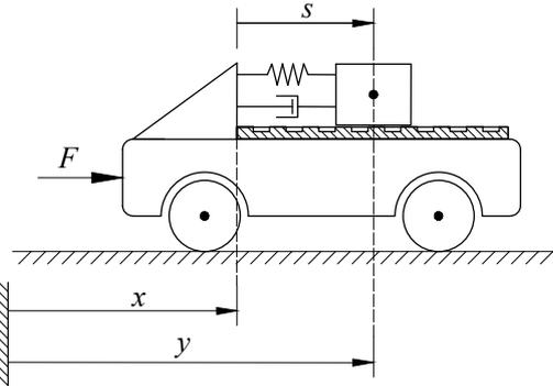
**FIGURE 9** Mass on car system with  $\alpha = 0$  rad.
