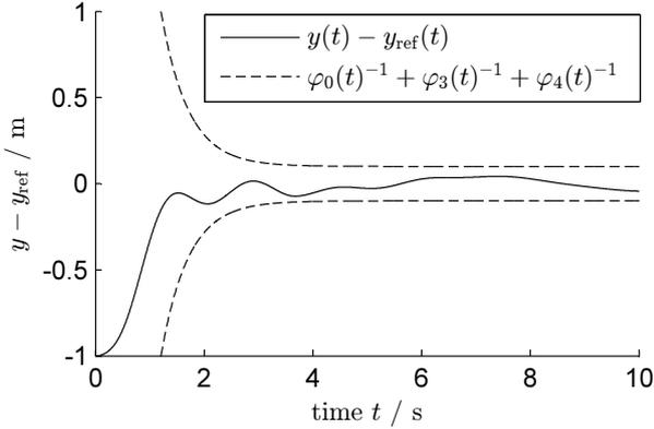
Fig. 10 a: Funnel and tracking error
