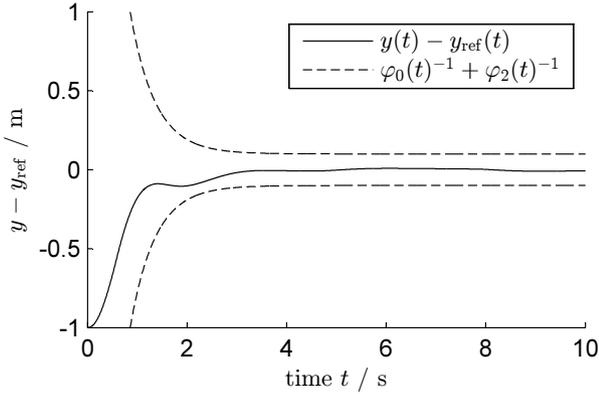
Fig. 8 a: Funnel and tracking error
