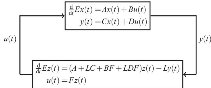
FIG. 6. Controller for regular systems.
