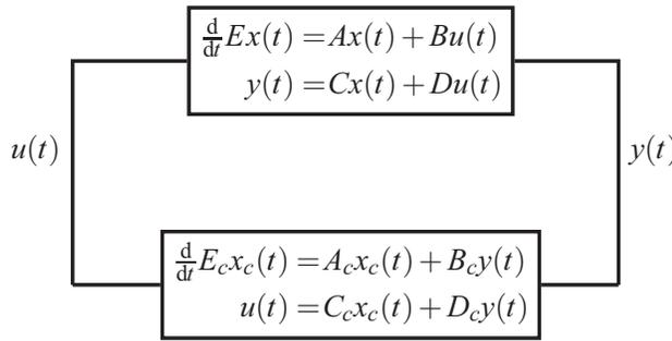
FIG. 4. Interconnection with a controller.
