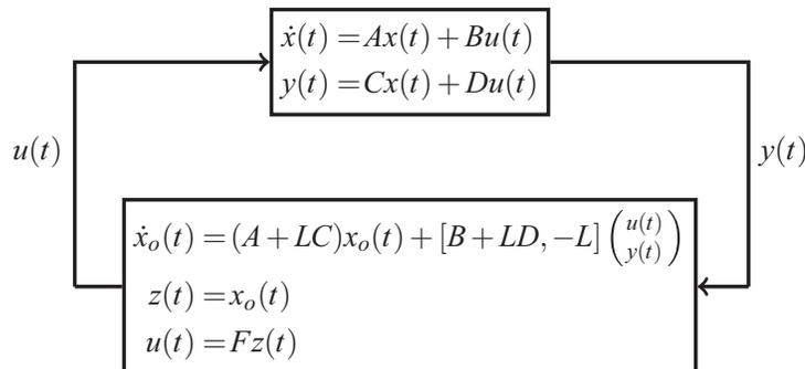
FIG. 2. Controller for ODE systems.
